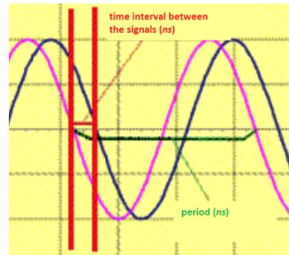
$$c = \frac{\Delta s_2 - \Delta s_1}{\Delta t_2 - \Delta t_1} = \frac{\Delta s_2 - \Delta s_1}{\Delta t_{c2} + \Delta t_w - \Delta t_{c1} - \Delta t_w} = \frac{\Delta s_2 - \Delta s_1}{\Delta t_{c2} - \Delta t_{c1}}$$
